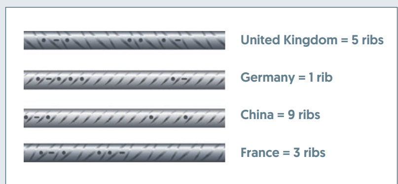
Figure 2: Determining country of origin of rebar. Source: ukcares.com
